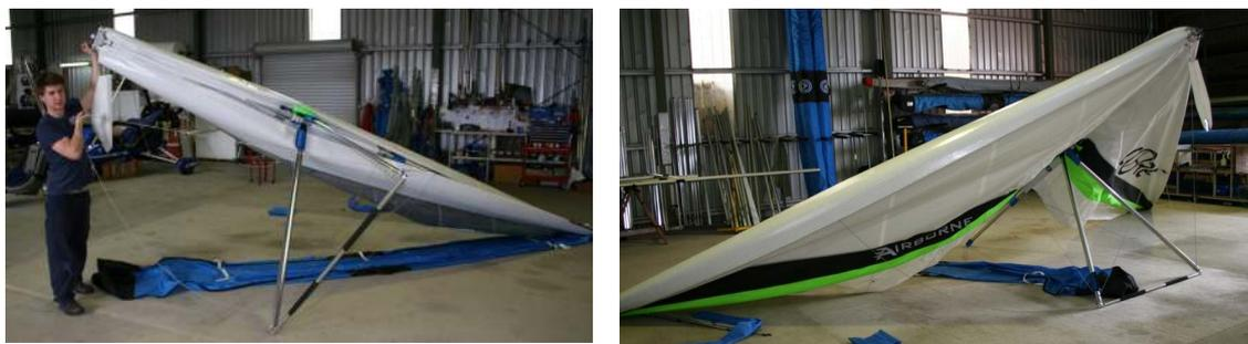
Figure 4 Standing glider on control frame and spreading wings
