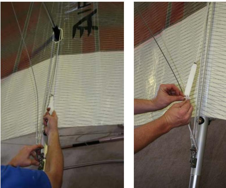
Figure 32 Tying pull back bungie and pulling tension
