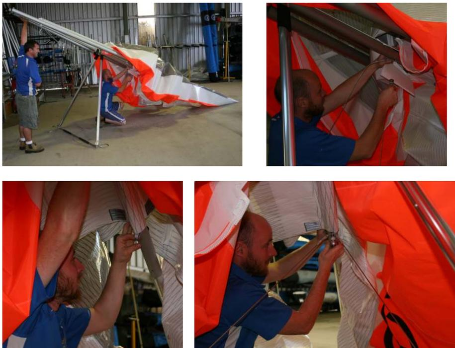
Figure 20 Sliding keel pocket into place
