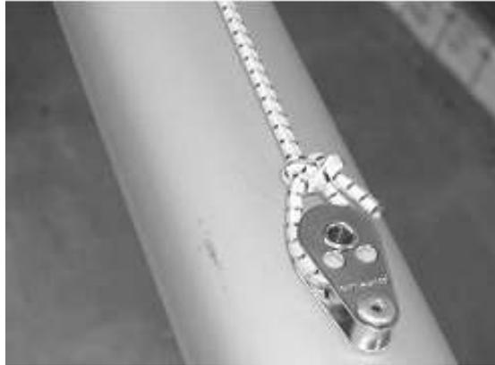
Figure 5 Removing pull back bungie
