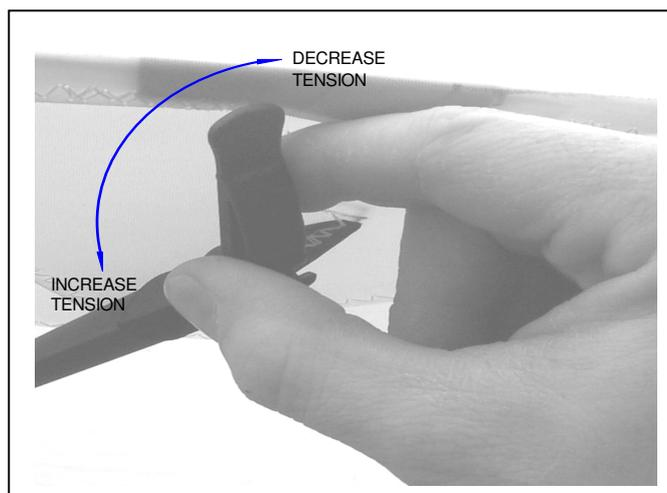
Figure 39 Adjusting Batten Tension
