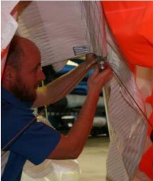
Figure 14 Removing Rear Wires
