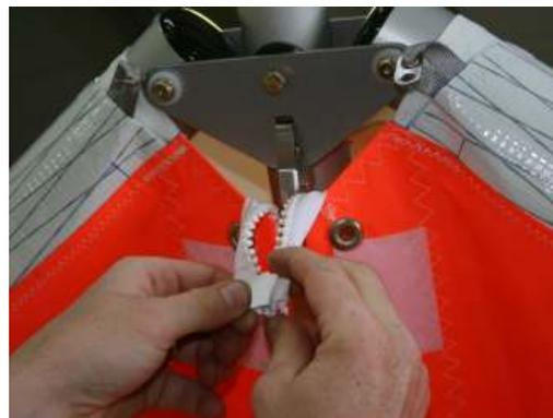
Figure 24 Fitting undersurface zipper
