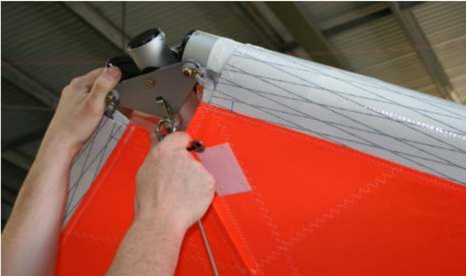
Figure 34 Attaching front bottom wires
