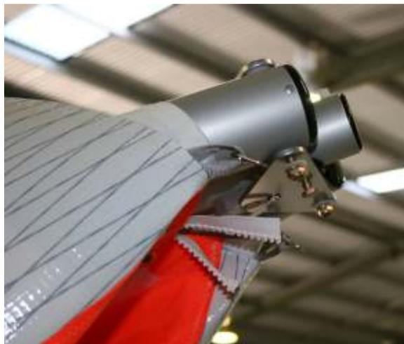
Figure 21 Sliding sail completely onto airframe
