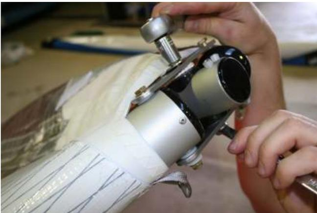
Figure 23 Fitting front top wire
