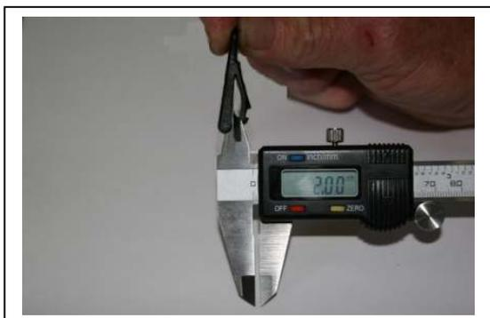
Figure 37 Batten End Fitting Dimension Check
