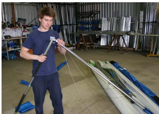
Figure 3 Assembling control frame
