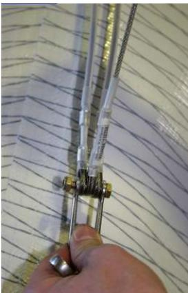
Figure 9 Removing rear top wire
