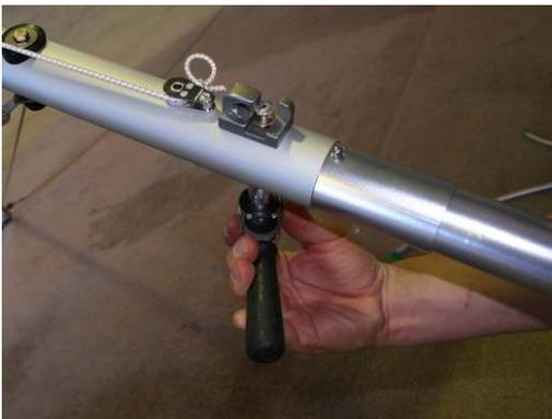
Figure 8 Removing pull back quick clip
