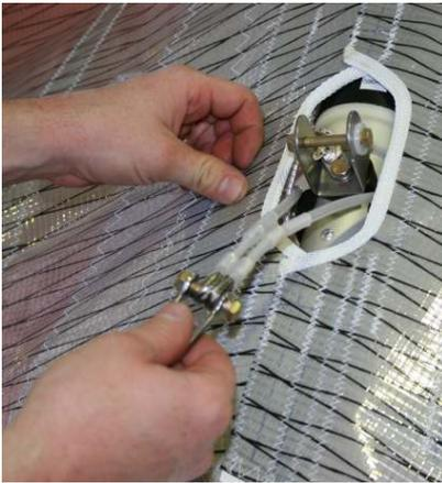
Figure 10 Removing king post
