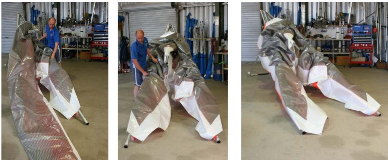
Figure 19 Sliding leading edges out the tips of the sail
