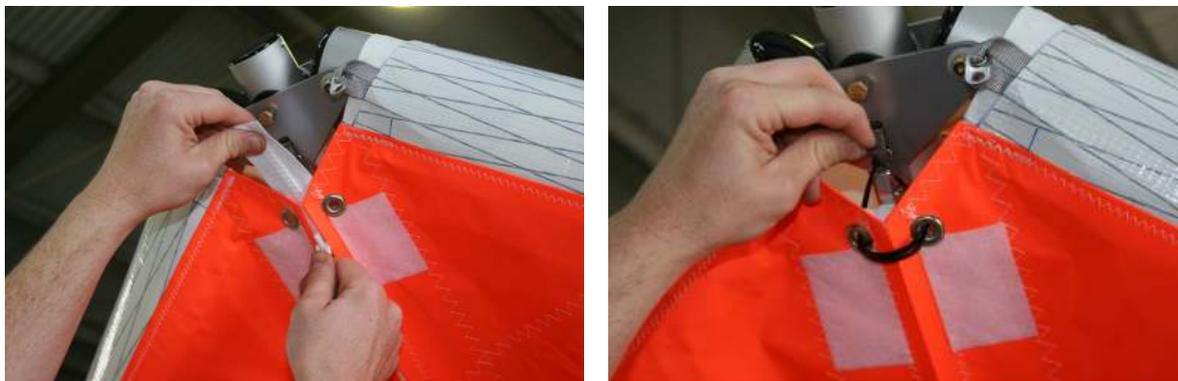
Figure 25 Fitting undersurface safety zip tie
