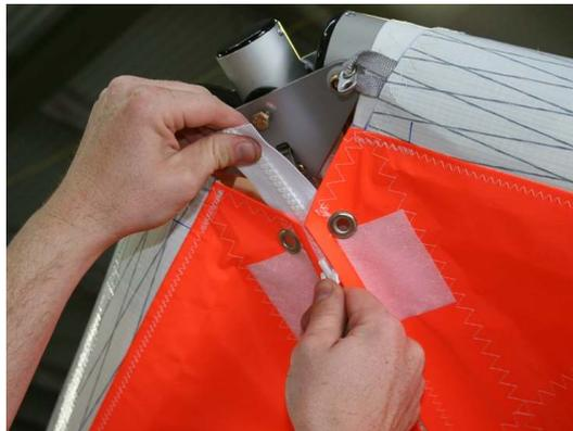
Figure 6 Removing zip tie and under surface zipper
