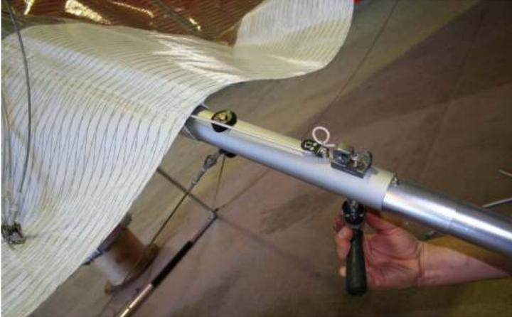
Figure 29 Fitting pull back quick clip
