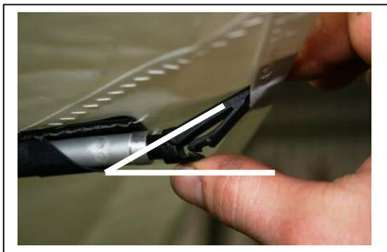
Figure 36 Inserted Batten End Unloaded Angle Check
