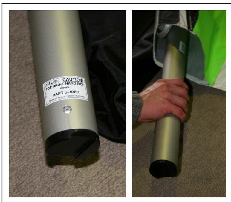
**Figure 1 Insertion of Rear Leading Edges**
