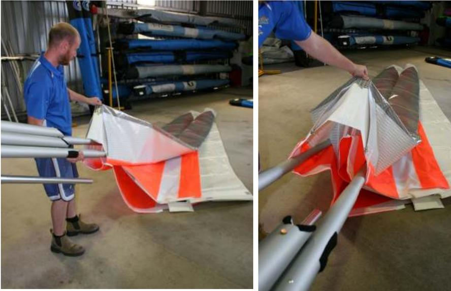
Figure 17 Sliding leading edges into sail
