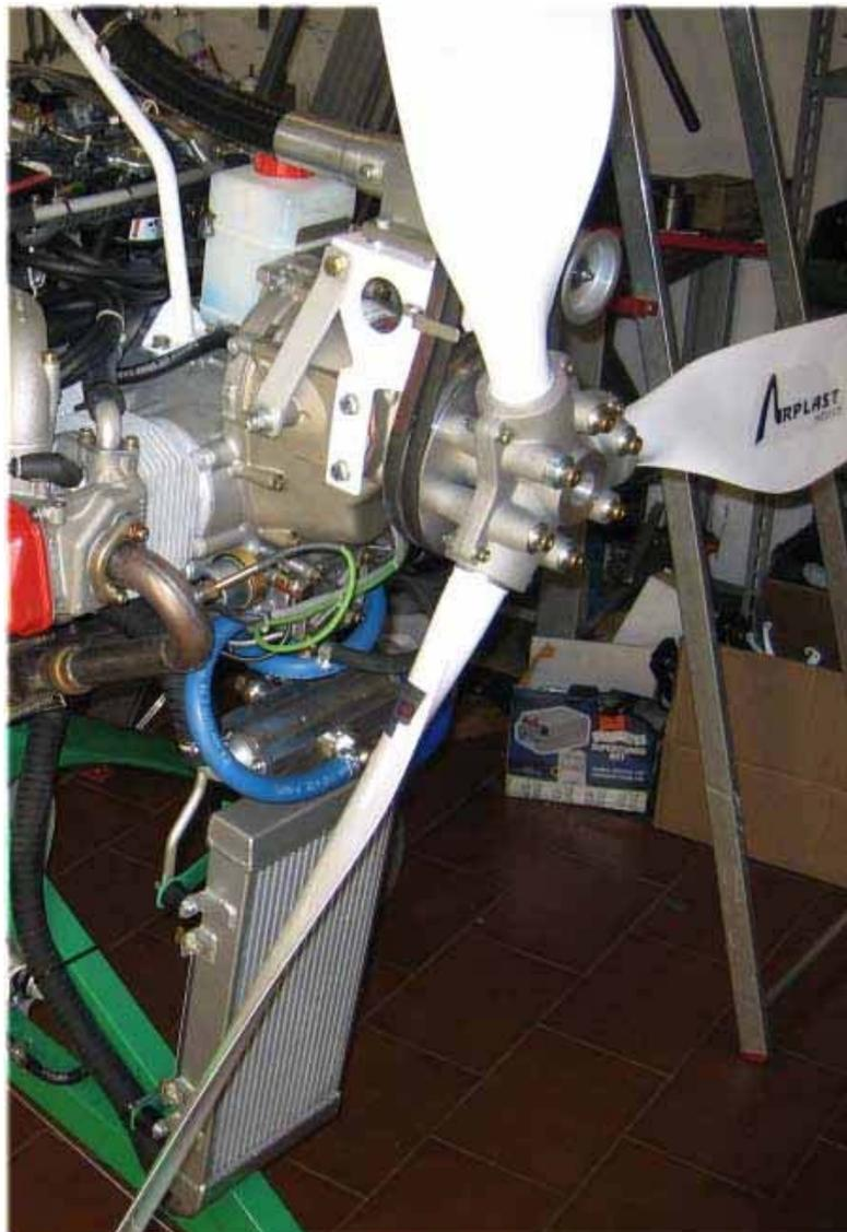
*Figure 2.10 – Three Bladed Propeller*
