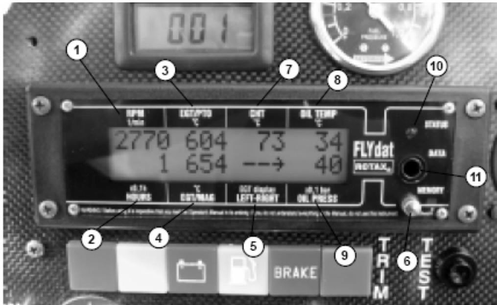
All the engine's instruments are grouped in the FLYDAT digital instrument supplied by ROTAX.
