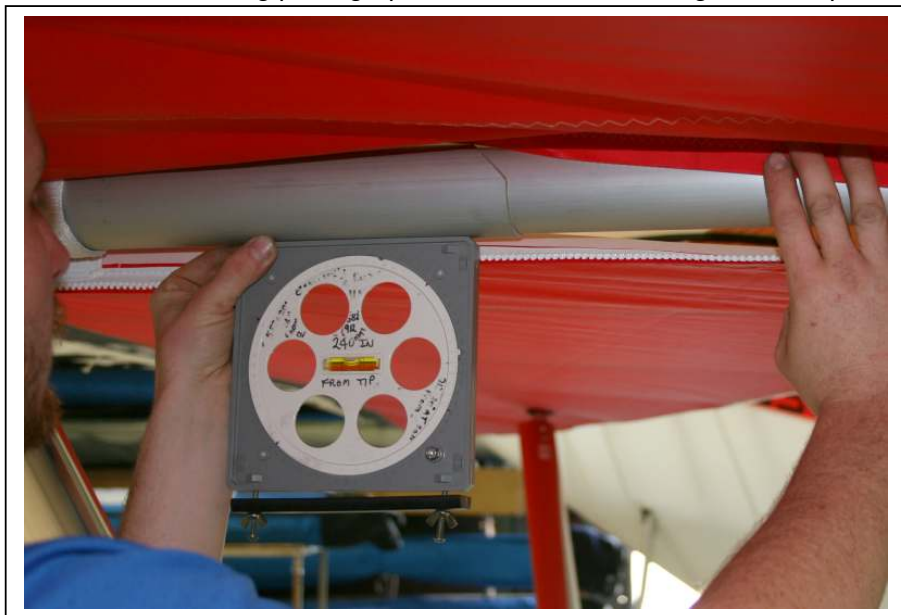
Figure 27 Setting Reference Keel Angle
