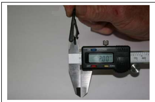
Figure 26 Batten End Fitting Dimension Check
