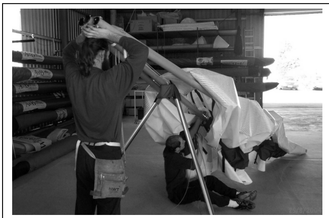
Figure 16 Position Keel Pocket Forward Of Rear Wires
