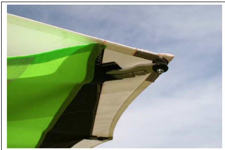
Figure 22 Locate Tip Over-Centre Battens
