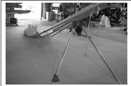
Figure 12 Frame Preparation for Sail Reinstallation
