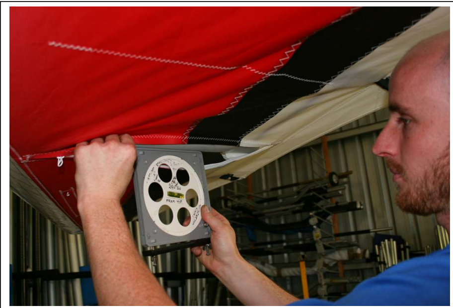
Figure 29 Checking the Outer sprog angle
