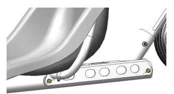
Base tube bolts and castellated nuts tightened until the saddles contact the channel only. Do not overtighten, split rings fitted.
