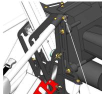
The front pole bolt and mast pivot bolt, wing nuts finger-tight, safety pins fitted.
