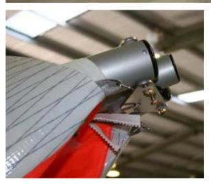
Figure 21 Sliding sail completely onto airframe
