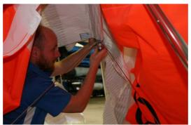
Figure 20 Sliding keel pocket into place
