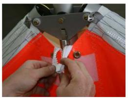
Figure 24 Fitting undersurface zipper
