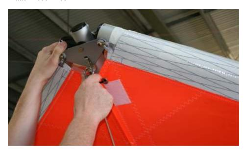
Figure 34 Attaching front bottom wires
