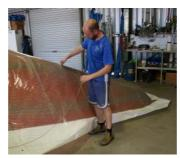
Figure 11 Removing top and bottom side wires
