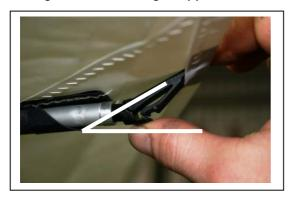
Figure 36 Inserted Batten End Unloaded Angle Check
