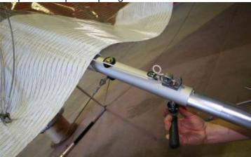
Figure 29 Fitting pull back quick clip
