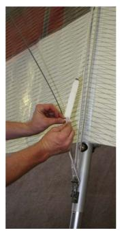
Figure 32 Tying pull back bungie and pulling tension
