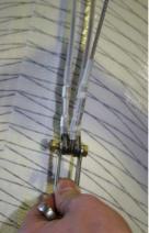
Figure 28 Routing pull back wires and attaching rear top wire
