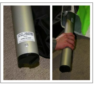
Figure 1 Insertion of Rear Leading Edges
