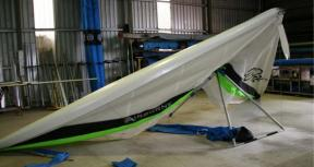
Figure 4 Standing glider on control frame and spreading wings
