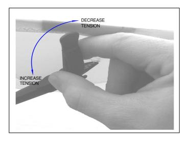
Figure 39 Adjusting Batten Tension
