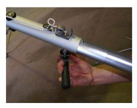
Figure 8 Removing pull back quick clip
