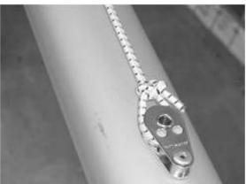
Figure 5 Removing pull back bungie
