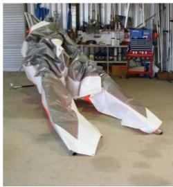
Figure 19 Sliding leading edges out the tips of the sail
