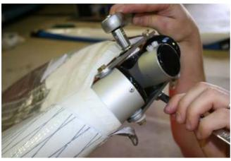
Figure 23 Fitting front top wire
