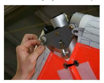
Figure 33 Attaching sail webbing tangs at the nose junction
