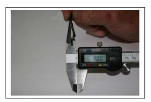
Figure 37 Batten End Fitting Dimension Check
