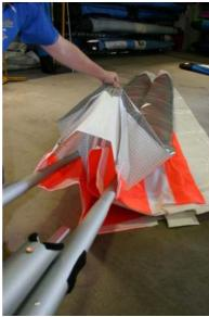
Figure 17 Sliding leading edges into sail
