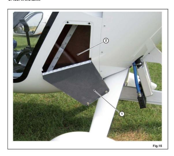
When refuelling it is imperative that the passenger door is fully open. In the event of a fuel spillage on the passenger door window, damage may occur to the transparency. Any fuel spillage on the cowling should be wiped off with a cloth.
