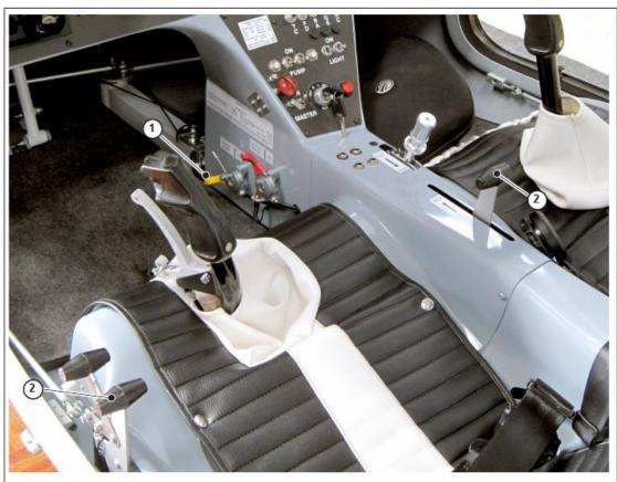
Fig.9 - Choke control lever
