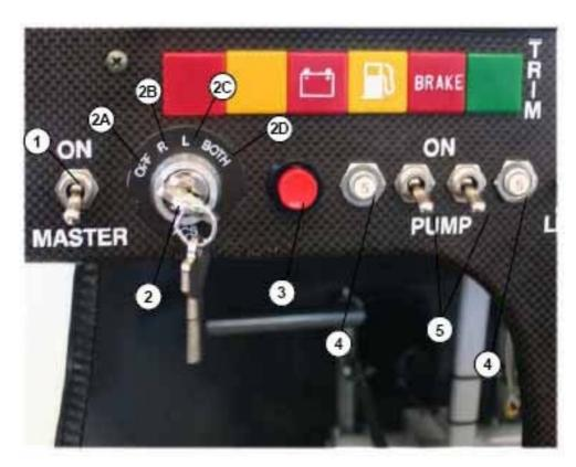
1 - Master SWITCH 2 - Ignition key 2A - OFF: Deenergized position 2B - R: Right magneto is on 2C - L: Left magneto in on 2D - BOTH: Both magneto are on 3 - Start push button - choke 4 - Fuel pumps circuit breakers 5 - Main - auxiliary pumps switch
