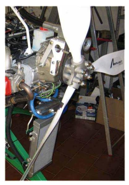
Figure 2.10 – Three Bladed Propeller
