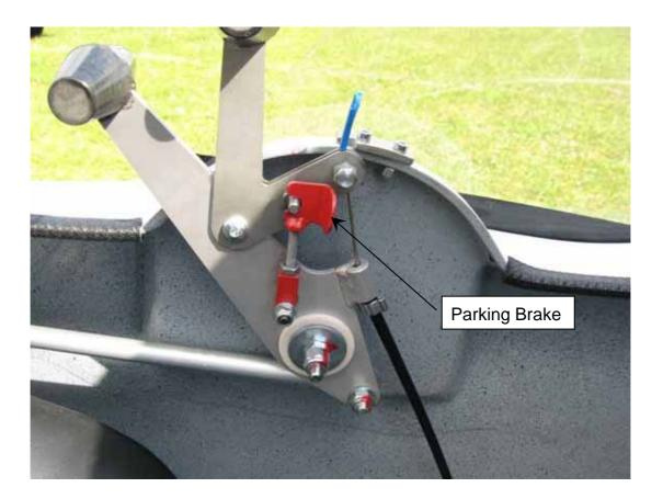
The lock is rotated to locate on the pin protruding from the main brake lever.
