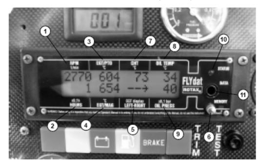
All the engine's instruments are grouped in the FLYDAT digital instrument supplied by ROTAX.
