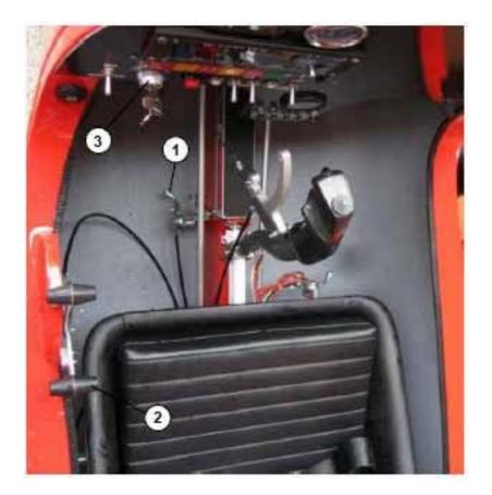
1 - Choke lever 2 - Throttle lever 3 - Ignition key
