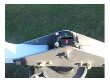
**Dispensation.** Gyroplanes manufactured by Magni Gyro Company and TAG Aviation that utilise the hub-bar design pictured above are exempted from the requirements of ASRA AD 2008.01. Testing and life of these hub-bars is as per manufacturer's recommendations or requirements. This dispensation is only applicable to hub-bar designs similar to that pictured.
