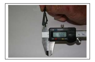
Figure 15 Batten End Fitting Dimension Check
