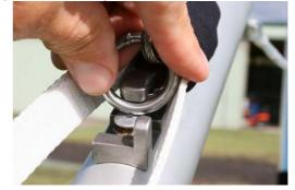
Figure 7 Section 5. Tensioning cross bar and shackle located in block
